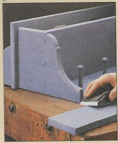
To give the Coat Rack a worn appearance, sand some of the edges after painting, and round the corners that would get the most wear. Then add a few dents and scratches.
