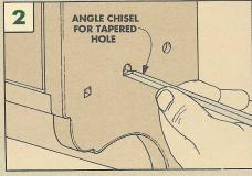
Next, square the screw holes with a chisel. The pegs will fit easier if you round their bottom edges with sandpaper. Finally, add glue and tap the pegs in place.
