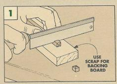
To make square pegs, first cut a  $\frac{3}{8}$ "-square piece to a rough length of 18". Then, using a disc sander, shape the end to a slight pyramid and cut the peg about  $\frac{3}{8}$ " long.
