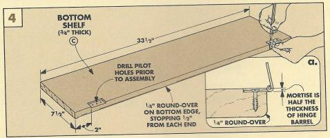
for the screws. Then, rout a 1/4" round-over on the front bottom edge, see Fig. 4a.
