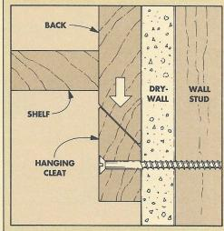
Here's how the hanging system works. A beveled cleat is cut to length so it fits easily into the opening in the back of the coat rack. Then the cleat is screwed to a pair of studs in the wall. After it's finished, the coat rack is hung on the cleat so the mating bevels interlock.
